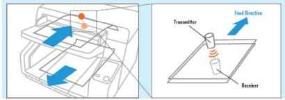
The center position sensor detects double-feeding and stops the scanner.
